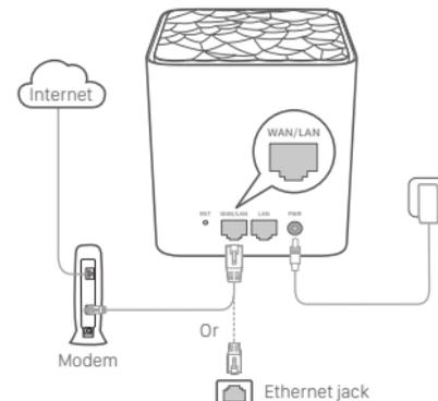
1. Power off your modem, and remove and reinstall its battery (if any).
