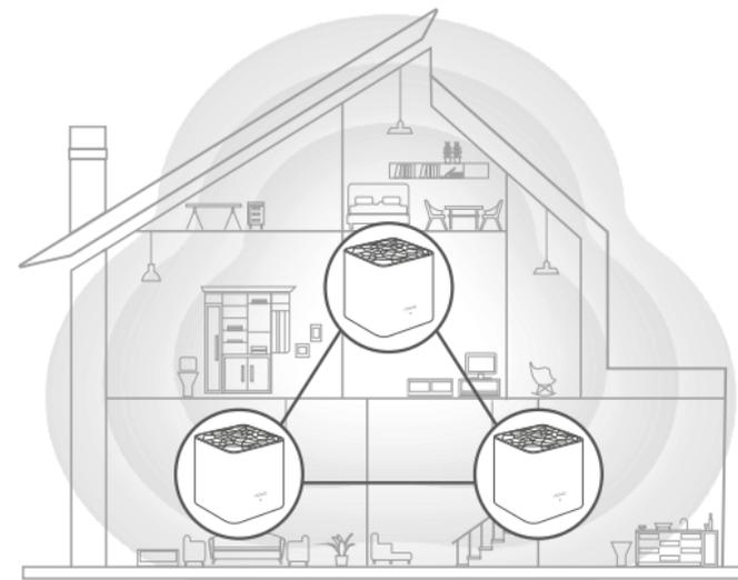
2. Use the other included power adapters to connect the remaining secondary nodes to power sources, their LED indicators light solid green. Wait about for 40 seconds. The secondary node is connecting to another node when its LED indicator blinks green.
